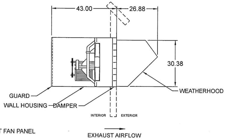
END VIEW DIMENSIONS ARE FOR HOUSING NOT FAN PANEL
